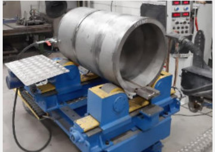
Using this system, roll-bent and submerged arc-welded components can be used as input material for our drum components as an alternative to centrifugal casting. The investment in the new system and the manufacturing processes significantly increase the flexibility and cost-effectiveness of rotor production for our decanters.
