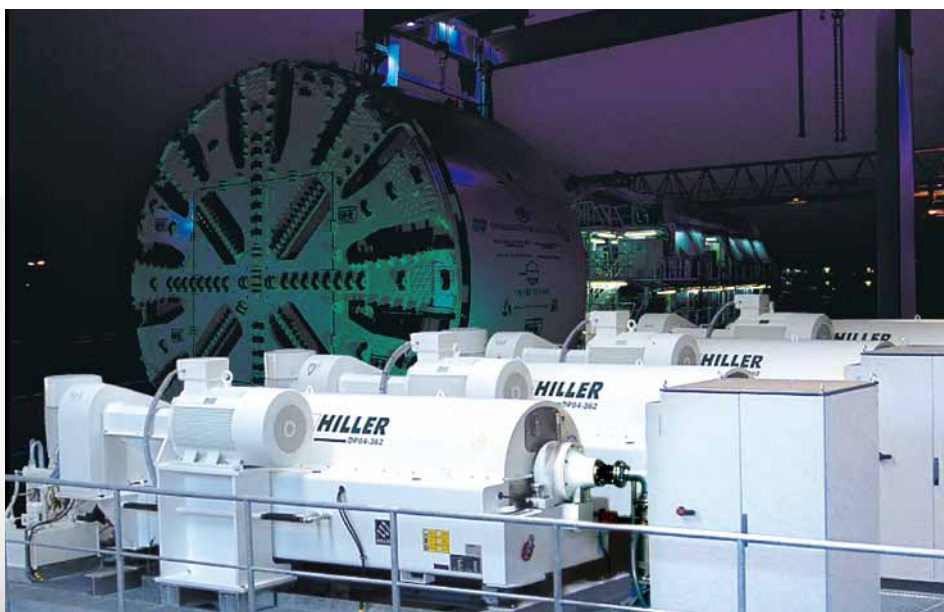
HILLER decanters in tunnel construction
