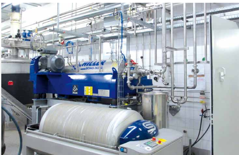
HILLER decanter in a chemical process
